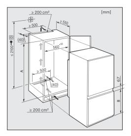
Before installing the appliance make sure the housing unit is the correct size. Specified ventilation gaps must be maintained in order to ensure that the appliance functions correctly.
